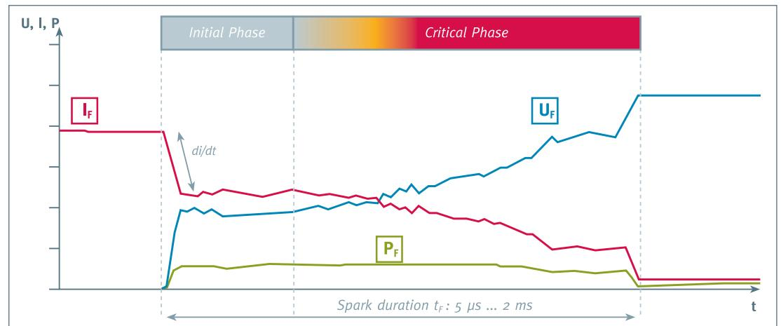
*Current, voltage and power of a spark interrupted by DART.*
