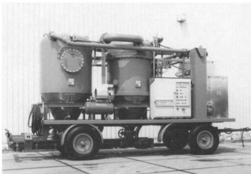
Figure 5-60 Large mobile vacuum cleaner for collecting combustible/exposable dusts in industry. Both the main vessel and the connecting ducts are designed to withstand internal explosion pressures of 9 bar(g). Power requirement 45-55 kW. From Eckhoff (2003).
