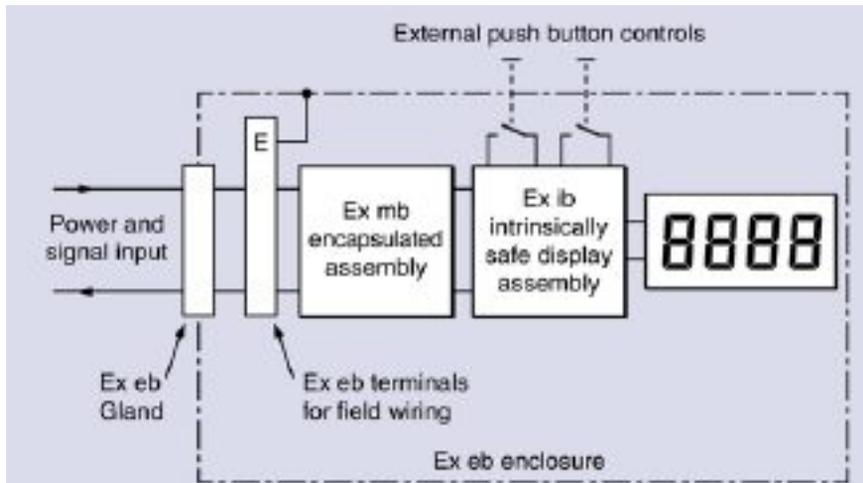
Figure 1 – Alternative Zone 1 instrument design
