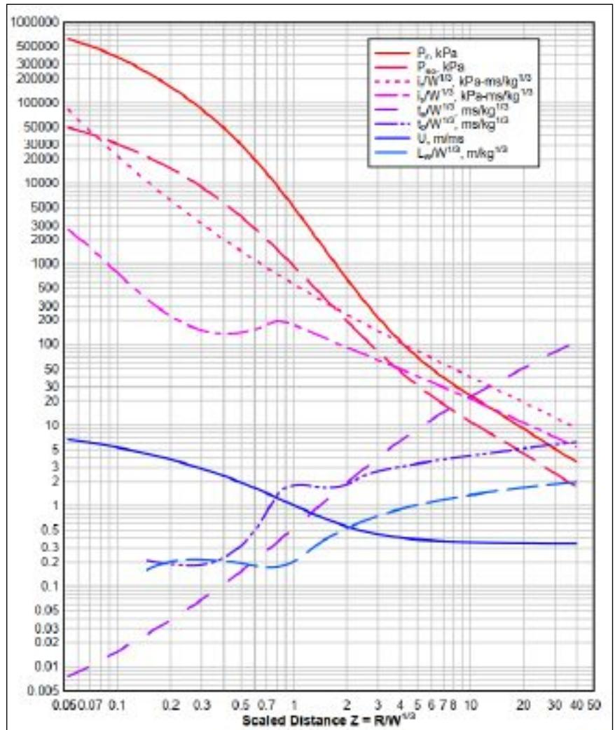
Figure 4 – Parameters of positive phase of shock spherical wave of TNT charges from free-air bursts<sup>[3]</sup>
