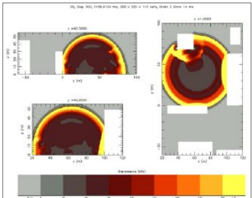
Figure 5 – CFD modelling of blast wave propagating against buildings (ProSAir<sup>[8,9]</sup>)
