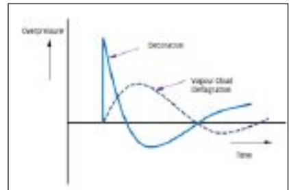
Figure 3 – Difference on Pressure Curve Characteristics: VCE vs. HE Detonation
