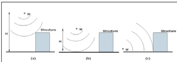
Figure 2 – Three types of unconfined blast - a) free-air burst; b) air burst; c) surface burst
