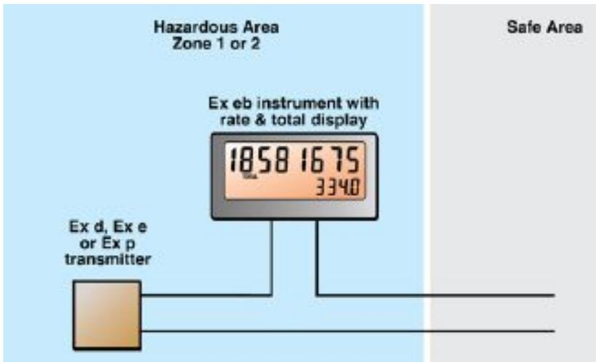
Figure 2 – Ex eb instrument can be safely connected to instruments with other types of explosion protection.
